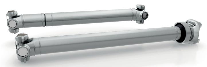
Select your Spicer for Scania replacement driveshaft components – or build your own driveshaft from Spicer components. Components to build Spicer driveshafts for Scania – from the U-joints to the tuber and more – are now available for the aftermarket.
